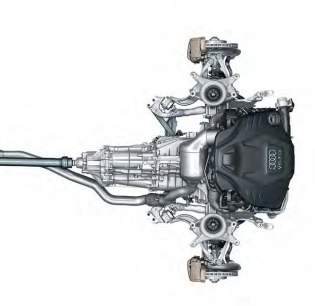
In the Audi A5 Coupé, asymmetric dynamic torque distribution continuously distributes drive power between the front and rear axles, depending on weather conditions, road surface and gradient. This leads to greater flexibility and an enhanced, sportier drive.
