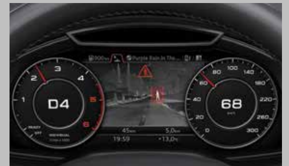
Image shows Audi Virtual Cockpit in classic view with optional Night vision assistant.
