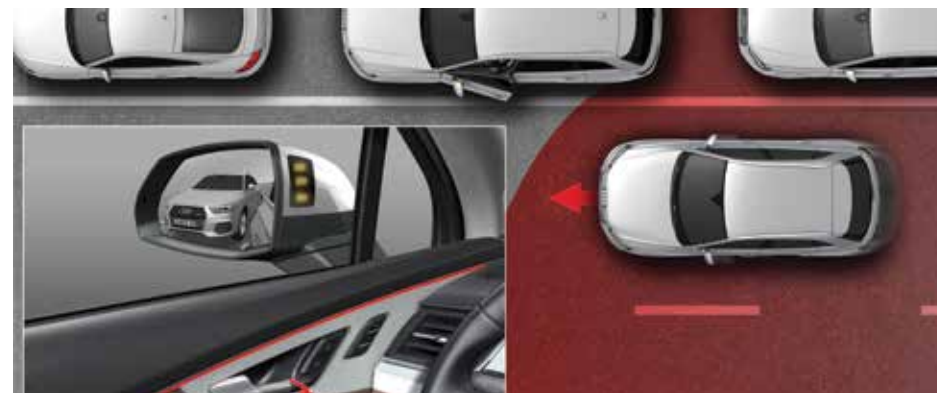
Exit warning featured in Parking pack advanced or Audi side assist including Pre-sense rear and exit warning
