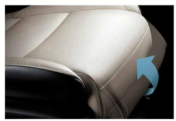
**Electric seat cushion extension ('3' and '4')** – Designed with long-legged drivers in mind, the seat cushion can be extended for optimal driving comfort.
