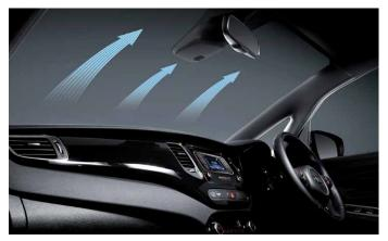
**Auto de-fogging system (new special edition 'SR7' upwards)** – A sensor automatically initiates a de-fogging process when condensation is detected on the windows to ensure optimal visibility and to prevent humidity from building up on the windows.
