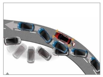
**ESC (Electronic Stability Control)** – if a loss of grip is detected, ESC applies the correct amount of brake pressure to each individual wheel, helping you maintain control and stability. It also reduces engine power to help you maintain control.
