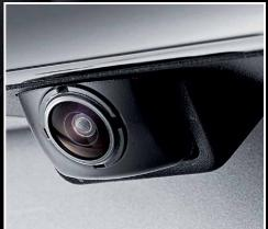
Reversing camera integrated into the centre fascia screen ('3' and '4' grades only) – The popular reversing camera feature is combined with reversing sensors which help minimise the collision risks involved when parking or manoeuvring. The rear camera view shows superimposed parking guidelines to assist the driver in easier, more effective parking. Reversing sensors are a standard feature on the new special edition 'SR7' models upwards.
