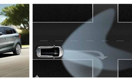
**Cornering lights** - When driving at night the cornering lights automatically turn on to illuminate potential hazards when turning.
