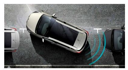
The Carens can even help you park your vehicle easily and conveniently with the Parallel Park Assist System (PPAS) ('4' grades) – This clever system searches for a parallel parking space via 10 sensors (6 at the front and 4 at the rear) and once found, calculates the optimum route to park the vehicle into the space. The steering wheel is operated automatically, therefore all the driver needs to do is select the appropriate gear displayed on the LCD display and control the accelerator and brake.
