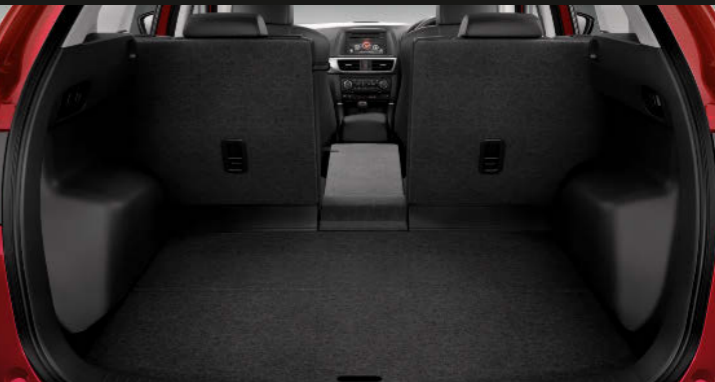
REAR INDEPENDENT FOLDING CENTRE SEAT Long objects can be loaded by folding the rear centre seat flat, even when passengers are seated on both sides. The tonneau cover can be conveniently stored in the sub trunk box (not shown).
