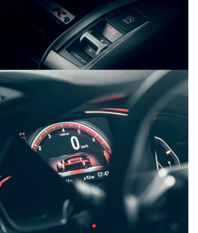
We have put the driver at the very heart of our thinking with a selection of driving modes: Comfort, Sport and track focused +R. Each mode sets the throttle response, the adaptive dampers, the steering force and feeling of the gear shift, to give the Type R three different personalities.
