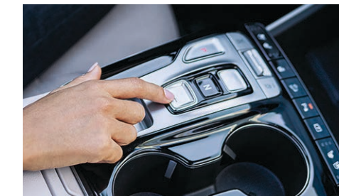
Electronic push button gear selection
