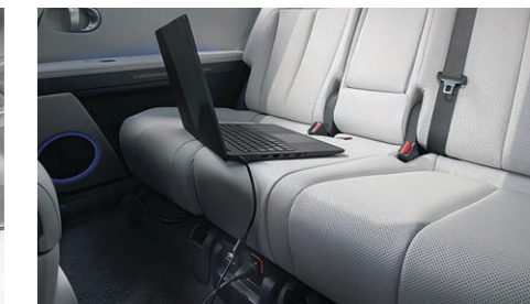
Vehicle-to-Load (V2L) two-way onboard charger
