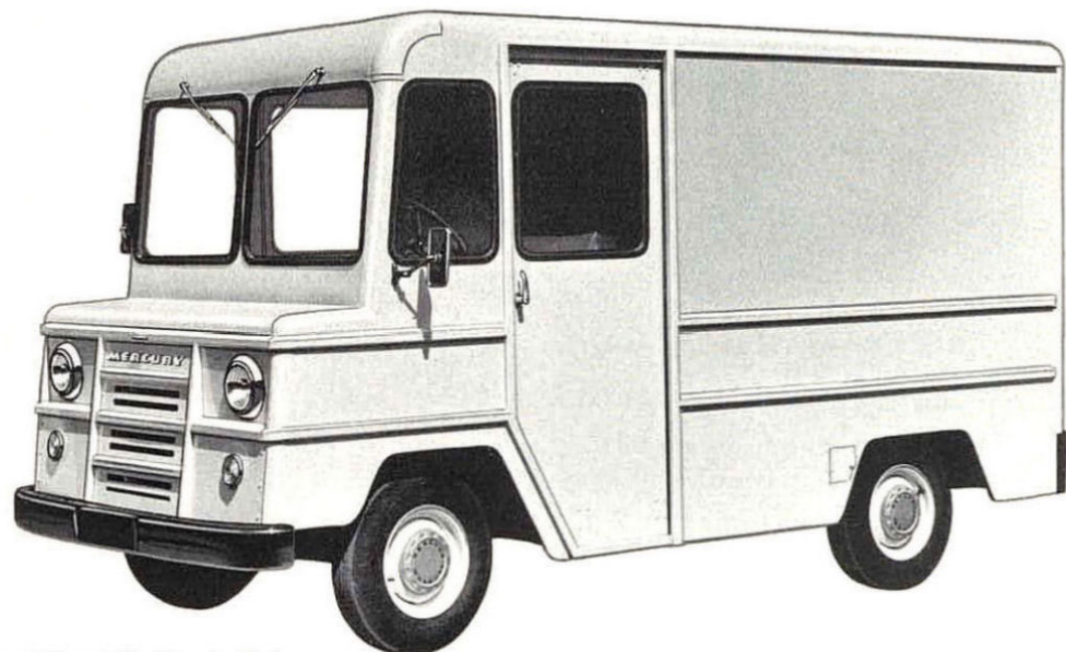
P-100 with 8-ft. body. Has 290 cu. ft. of load space on 102" wheelbase. Maximum GVW is 5,000 lb.
