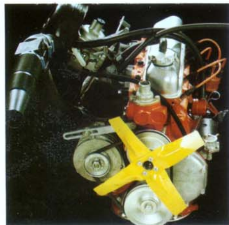
The two-litre B20 engine with outputs of 90 or 118 b.h.p. SAE.
