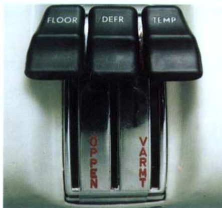
Thermostat-controlled heating system with clearly marked and illuminated controls.
