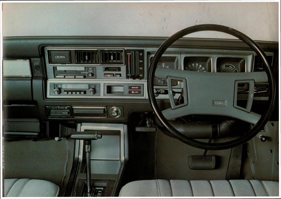
The radio is MW/LW/FM stereo push-button and self-seeking. And incorporated as an integral unit is the auto-reverse stereo cassette player which allows you to select either side of a tape at the touch of a button. The aerial uses
