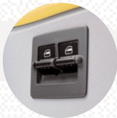
The standard front electric windows include obstruction sensors for added safety.
