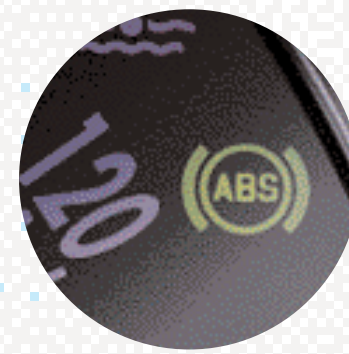
ABS helps you to steer around potential hazards, under hard braking, by preventing the wheels from locking.
