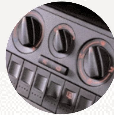
The optional CFC-free air conditioning has an air circulation switch to boost performance.
