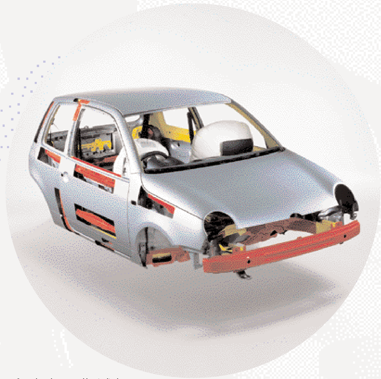
Strengthened square and longitudinal rods ensure greater stability.
