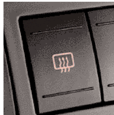
To conserve energy, the heated rear window automatically switches off after 15 minutes.
