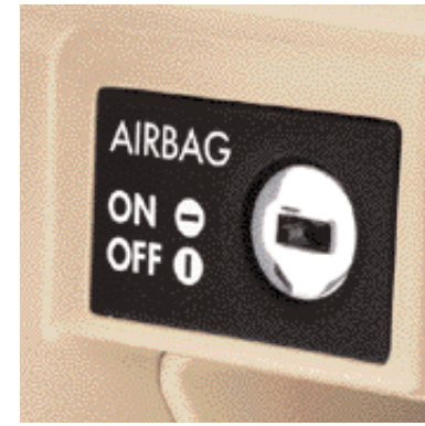
If you wish to fit a child seat in the front passenger seat, the passenger airbag must be deactivated. This option allows fast deactivation using the ignition key.
