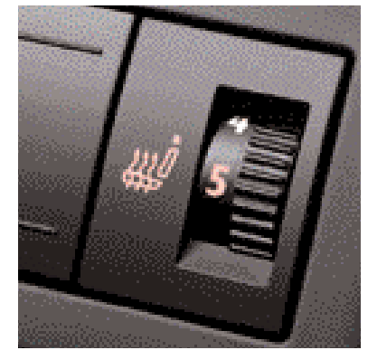
Front heated seats have five separate preset temperature controls. Available as part of the Winter pack on all models.
