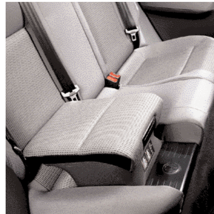
An integrated child seat is the fast and simple way to accommodate children between 3 to 6 years.
