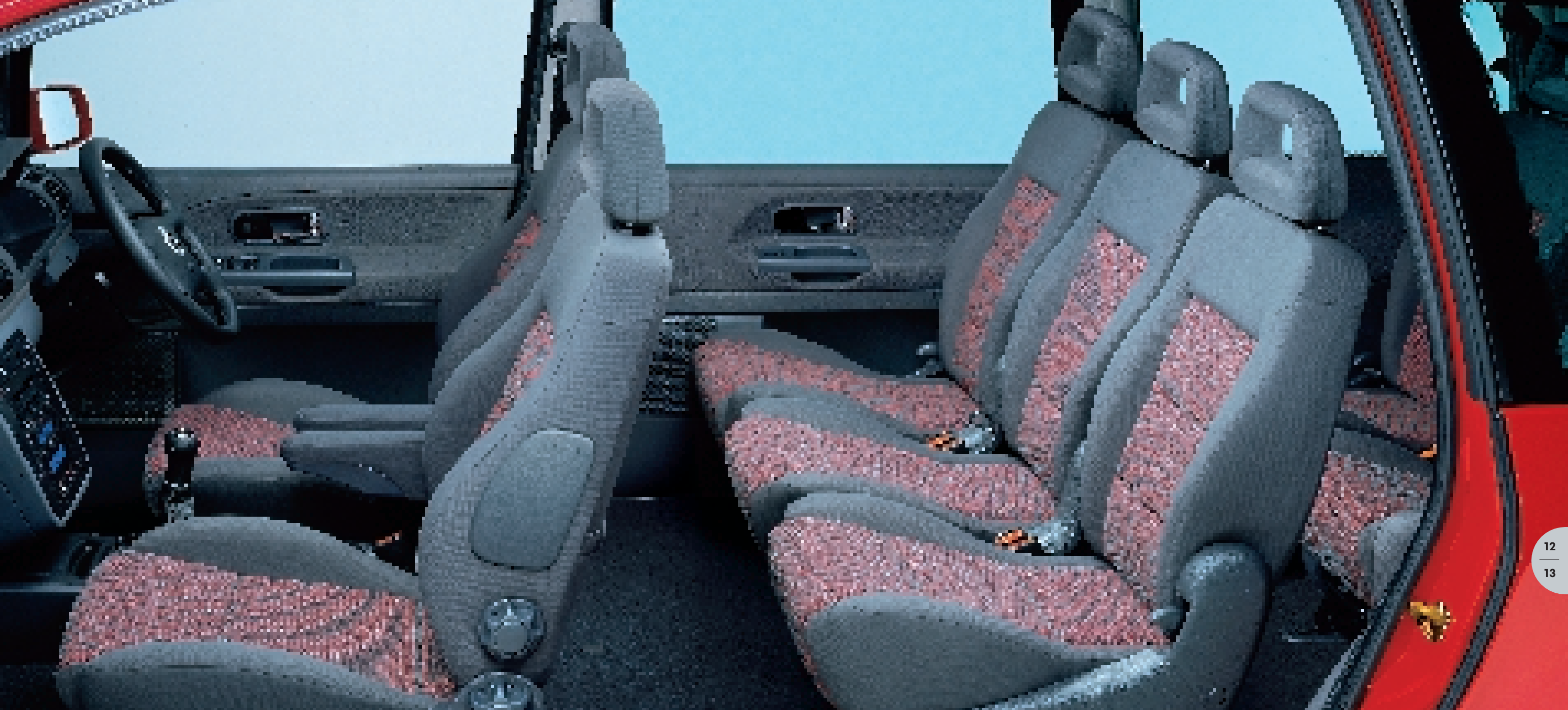
The middle row of three seats folds down to allow easy access to the two rear seats. Model shown is the Sport fitted with optional front and rear electronic climate control and ESP.
