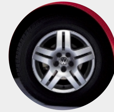
The elegant 'Avus II' 15" alloy wheels are available for the E, S and SE models. They are fitted with 195/65 R15 tyres and anti-theft wheel bolts.
