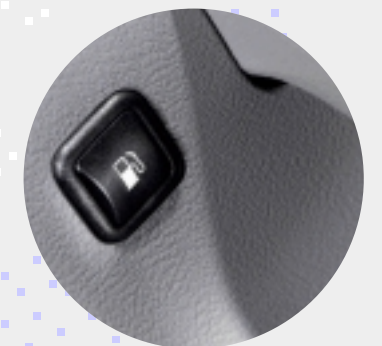
The fuel filler flap is opened via a button on the centre console.
