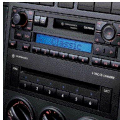
Standard on Sport models, a dash-mounted CD autochanger holds six discs.
