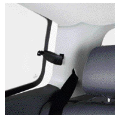
Manual rear vent windows provide draught-free ventilation (three door models only).
