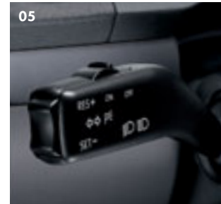
05 Cruise control can be set at speeds over 19 mph to maintain a constant speed. So even on long journeys you can have a high degree of relaxation. Optional on S, Sport, GT, GTI and R32 models.
