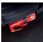
Powder type fire extinguisher
