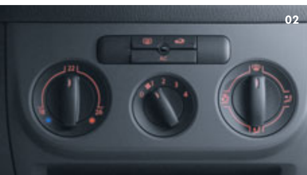
02 'Climatic' air conditioning with semi-automatic control produces a pleasant, consistent temperature throughout.
