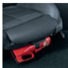
Powder-type fire extinguisher
