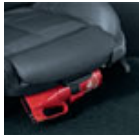
Powder-type fire extinguisher
