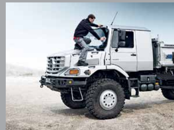
Non-slip steps and stand-on plates in the engine bay
