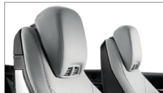
Thanks to Aircap's neck-level vents, front seat occupants can enjoy chill-free open-top motoring even in cooler weather
