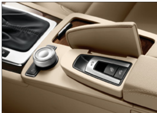
The soft-top release lever is concealed within the handrest for the central controller
