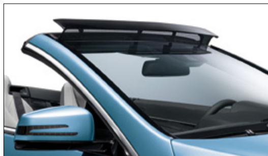
Aircap includes an electrically operated wind deflector fitted to the front windscreen surround
