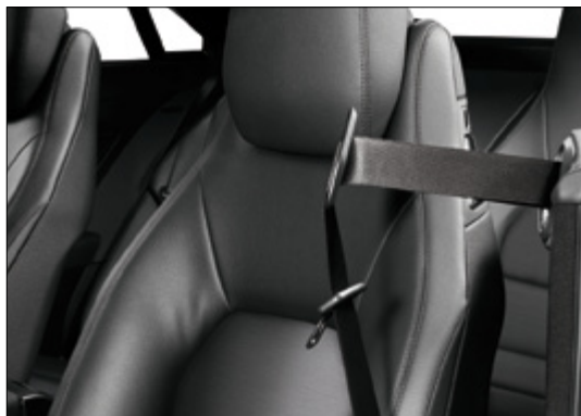
The automatic seat belt hand-over system brings the front seat belts within easy reach
