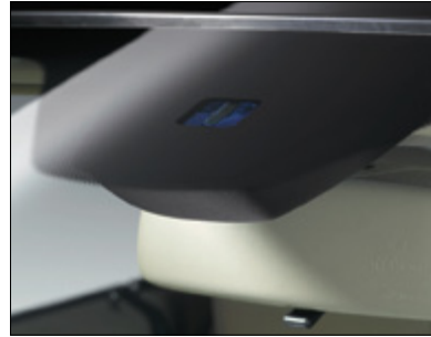
Rain sensor and light sensor for the Active Light System
