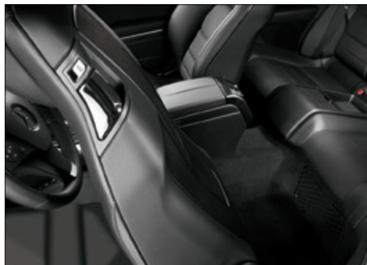
The Easy-Entry system enables the front seats to slide forward for better access to the rear
