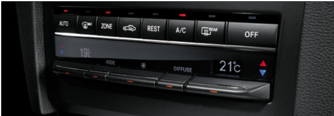
Luxury automatic climate control allows those in the front and rear to select different temperature settings
