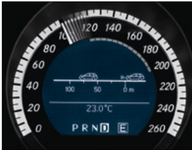
DISTRONIC PLUS radar-assisted cruise control
