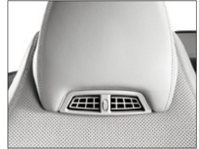
Airscarf neck-level heating system for Cabriolet
