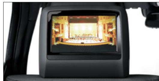
The two displays for the Rear Entertainment System are integrated in the front-seat head restraints
