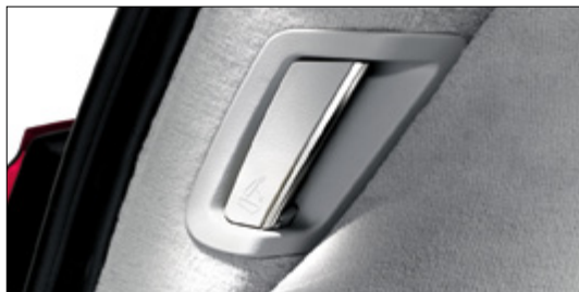
The Easy-Pack Quickfold lever on the D-pillar lets you fold the rear seats forward from the load compartment
