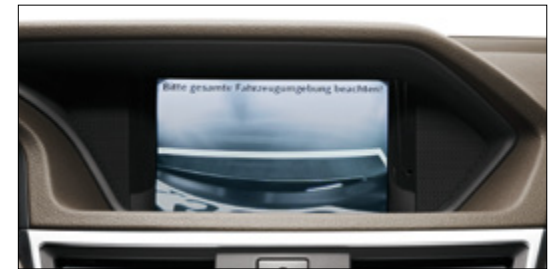
The reversing camera's wide-angle lens captures the area immediately behind the car
