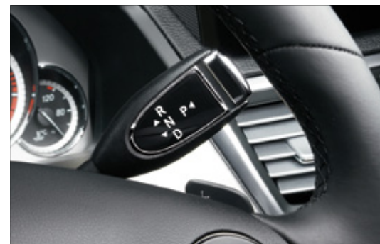
On V6 and V8 models, the transmission is operated via the Direct Select lever on the steering column
