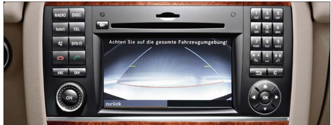
The reversing camera captures the area immediately behind the car
