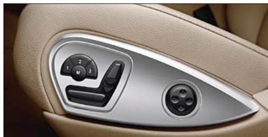
Individually stored seat positions can be called up at the touch of a button
