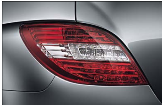
Tail lights featuring LEDs and fibre-optic technology
