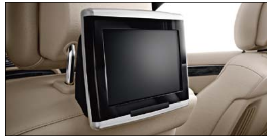
The displays for the rear seat entertainment system are mounted on the backs of the front seat head restraints
