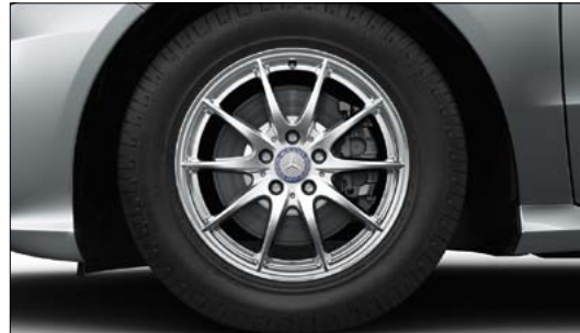
17" 10-spoke alloy wheels with 235/65 R 17 tyres (standard on R300 CDI BlueEFFICIENCY, code 25R)
