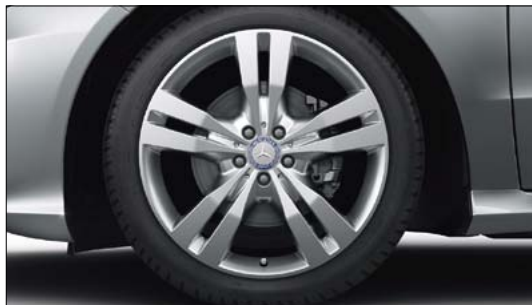
20" 5-twin-spoke alloy wheels with 265/45 R 20 tyres (optional, code R33; standard with Sports Styling Package)
