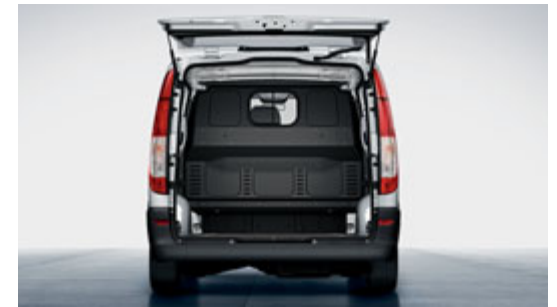
Wide-opening tailgate. Standard for models with standard roof: a tailgate with a wide opening angle of approx. 90°
