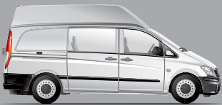
Vito Long: short wheelbase, vehicle length: 5008 mm, with normal-height roof or high roof
