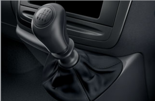
Practical gearshift. Shift/selector lever with ergonomically designed gear knob and artificial leather gaiter
