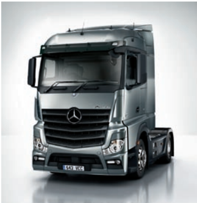
The StreamSpace cab has been specially optimised for low consumption. With a width of 2300 mm, an optional level floor and its 1.97 m headroom 1) it helps ensure greater economy in national and international long-distance transport – without having to relinquish any comfort
