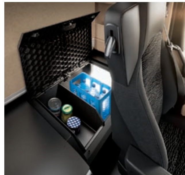
With a stowage capacity of up to 420 l the two stowage compartments under the bed offer plenty of room even for bulky items. They are accessible from both the inside and outside. As an option two sliding and removable stowage trays can be included for smaller items of equipment so that better use can be made of the space available
