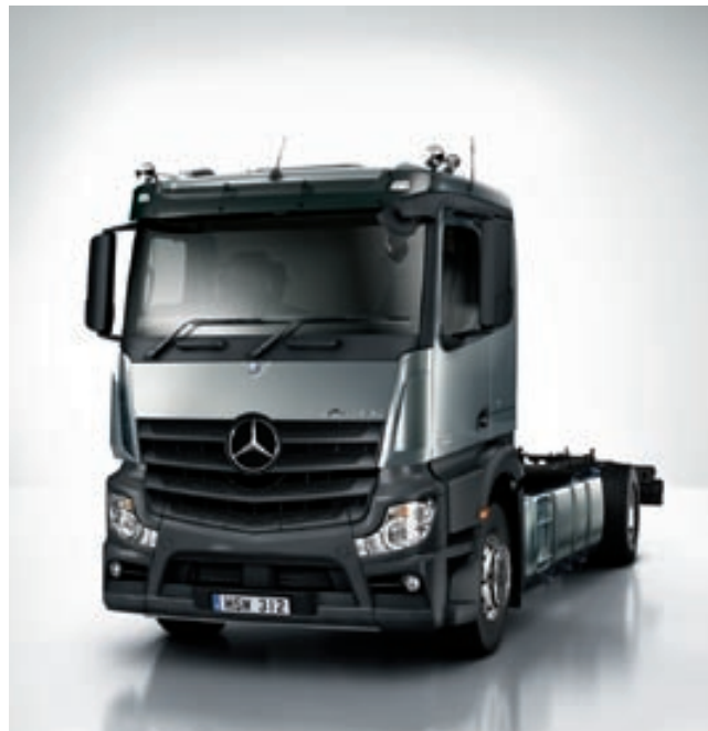
The ClassicSpace cab has a width of 2300 mm and an engine tunnel with a height of 170 mm or 320 mm. It is characterised by its excellent suitability for operating profiles in regional long-distance transport
