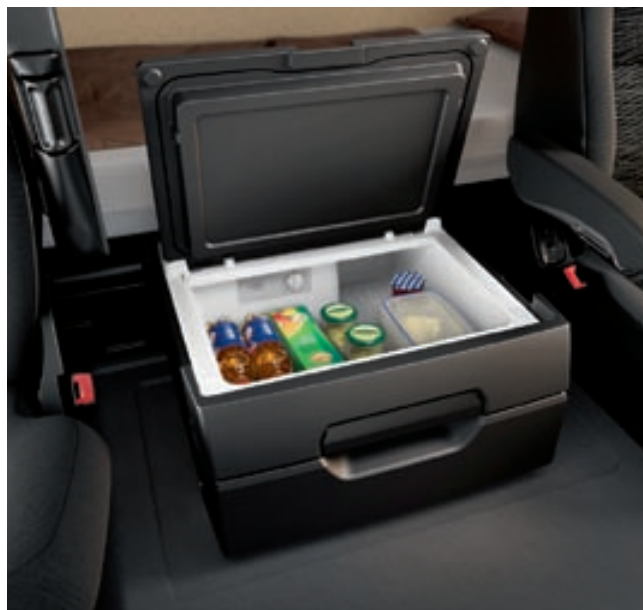
In cabs with an engine tunnel a practical drawer with a capacity of 51 l is housed in the centre section beneath the bed. As an option a refrigerator with a capacity of 26 l is also available
