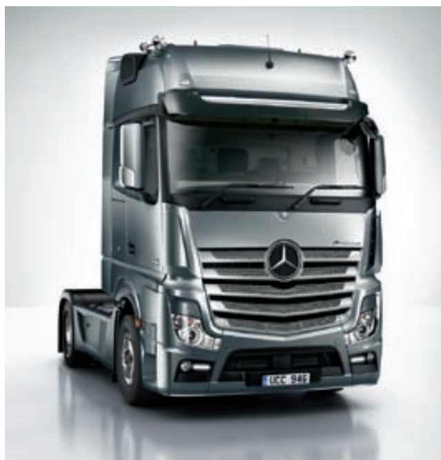
The GigaSpace cab: with a width of 2500 mm, a level floor throughout and headroom 1) of 2.13 m, it is the largest and most comfortable cab for the new Actros and meets the requirements of international long-distance transport in every respect
