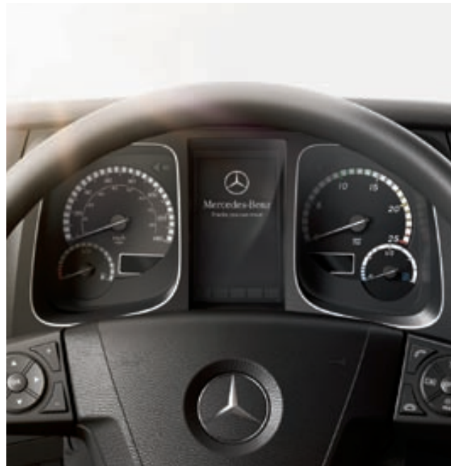
The new instrument cluster with a graphics-capable 10.4 cm TFT colour display adds tangibly more ease of operation. A variant with a 12.7 cm TFT colour display can be ordered as an option
