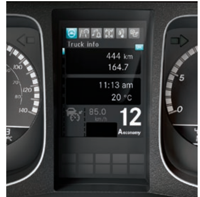
Thanks to the simple, intuitive menu navigation, the new, non-reflective instrument cluster shows all the important information quickly and easily. Numerous settings can also be adjusted here. Operation is via the buttons on the new multifunction steering wheel
