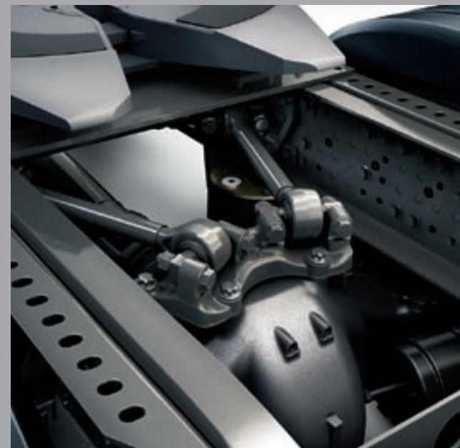
Innovative rear axle guide 1) : instead of a conventional wishbone, two longitudinal control arms whose operating lines' point of intersection is behind the drive axle are used in the new Actros. This results in better directionality, tangibly better understeer/oversteer characteristics and more transverse stability. More about this on pages 42/43
