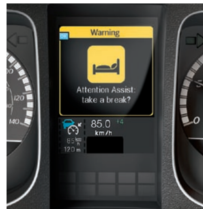
The new Attention Assist system, which is available as an option, can detect signs of increasing tiredness and inattention. It can issue a visual and audible warning sign and recommend the driver takes a break
