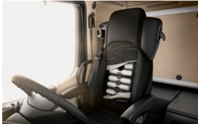
The comfort suspension seat and the climatised suspension seat with a massage function are available to prevent tension. Seven air cushions are inflated and then deflated again one after the other, producing a wave running from bottom to top which massages the driver's back
