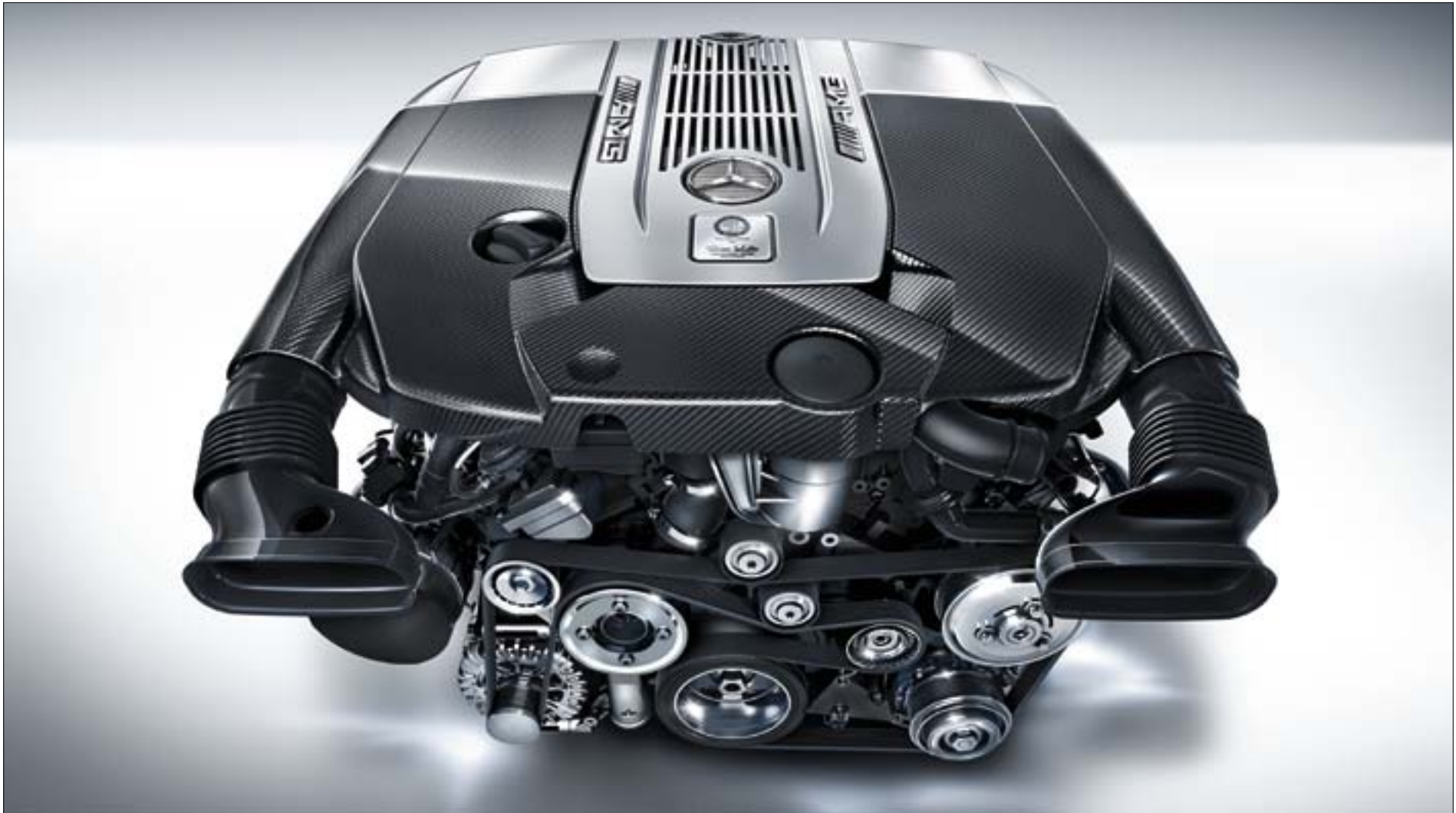
The AMG 6-litre biturbo V12 generates 630 hp (463kW) and 1,000Nm of torque
