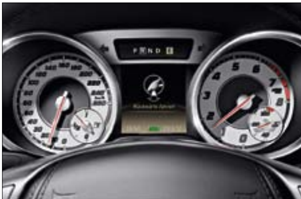
Speed Limit Assist shows you the current legal limit on the instrument panel and in COMAND Online's central display
