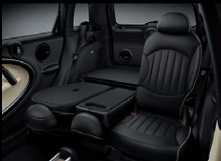
5. MINI Countryman backrest with a 40:20:40 split. Sections can be tilted and folded down separately
