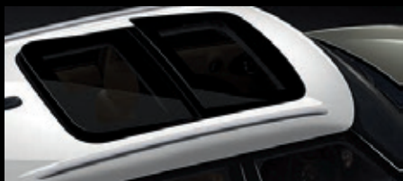
2. Panoramic glass sunroof – MINI Countryman, adjusted from the front and the rear
