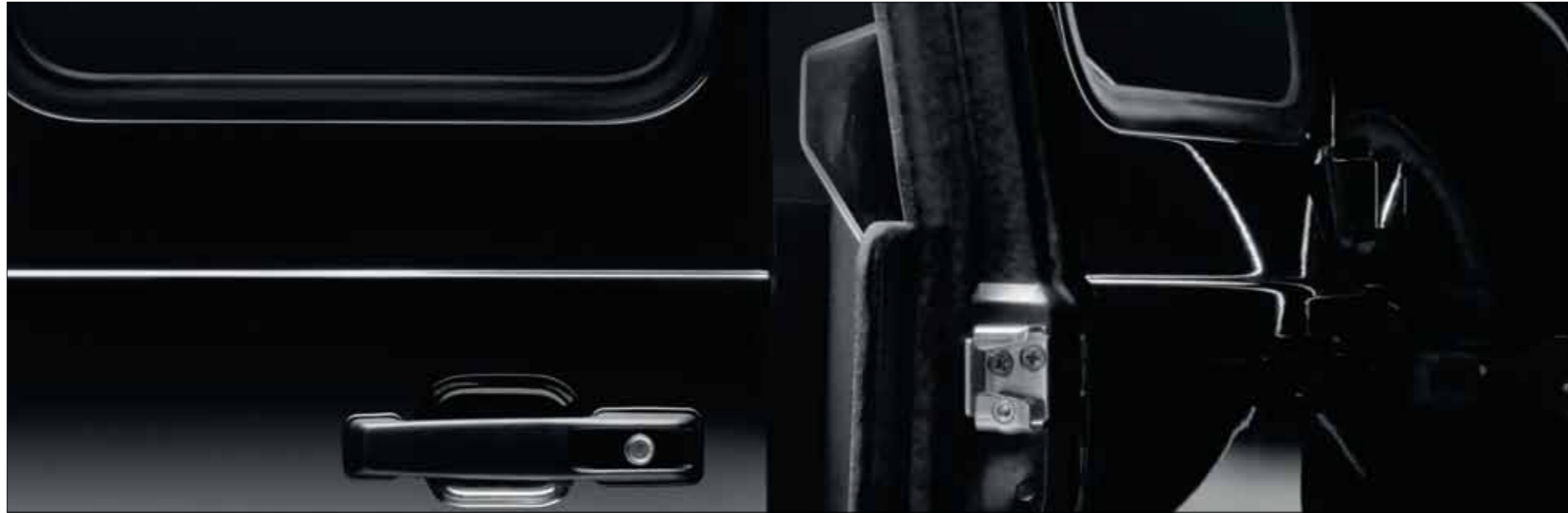
Strong at so-called weak points: where different materials come together, overlapping designs are used as a labyrinth system
