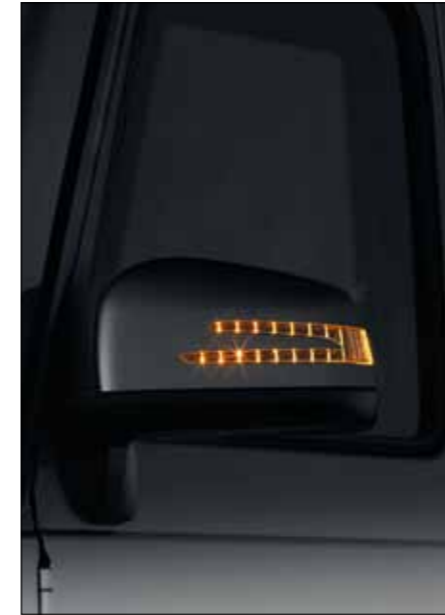
Flashing exterior mirror with built-in microphone for communications
