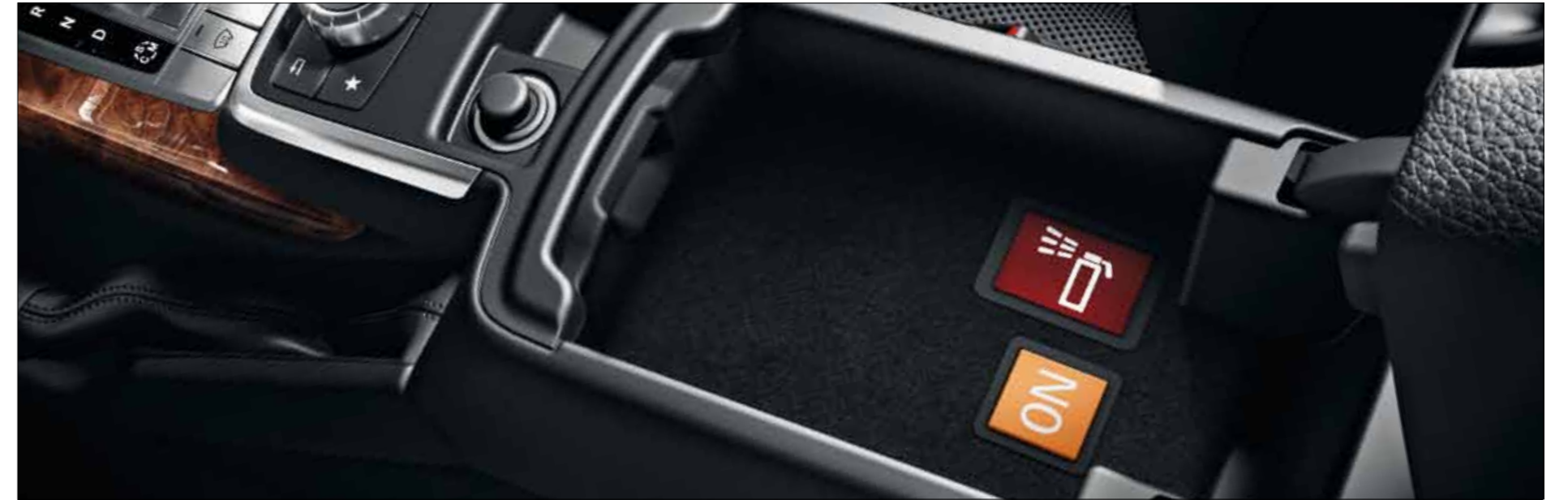
Because every second counts: the release button for the fire extinguishing system with strong signal effect
