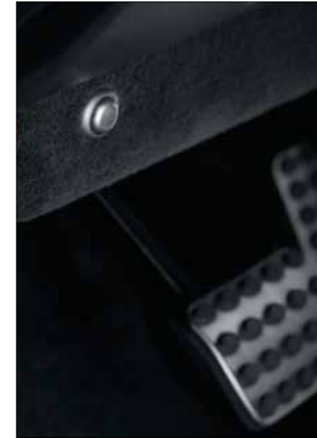
The driver's trigger for the at-risk alarm system near the steering wheel
