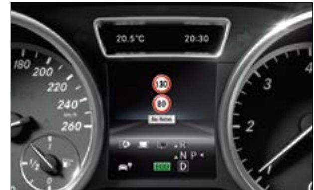
Speed Limit Assist alerts you to the current legal limit on the instrument panel and in COMAND Online's central display
