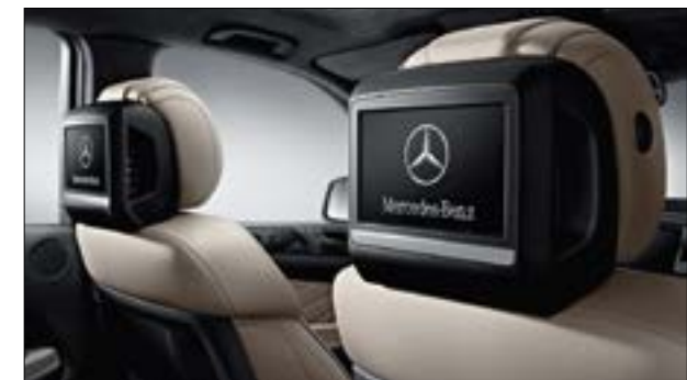
The rear seat entertainment system colour displays are attached to the backs of the head restraints
