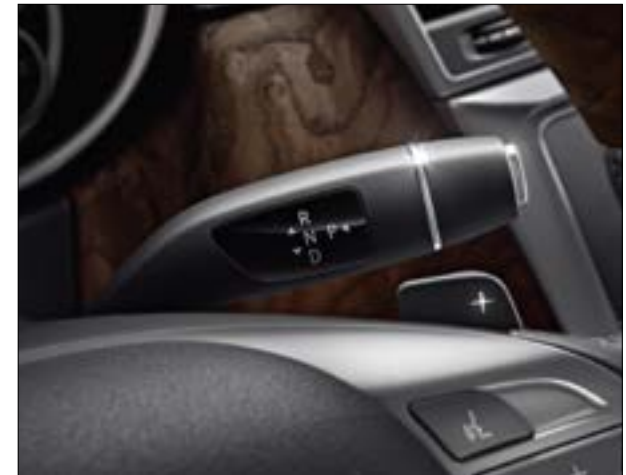
Transmission operation with the Direct Select lever: you can also control gear changes via the gear shift paddles on the steering wheel
