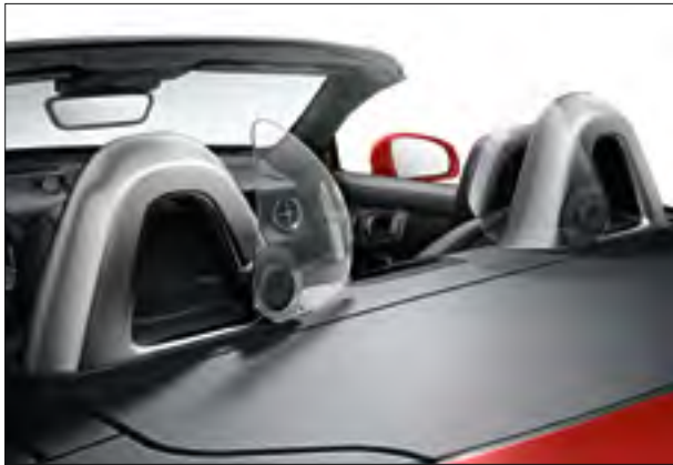
Airguide wind deflector, comprising twin Plexiglas® panels
