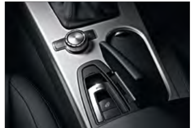
Roof controls and central controller
