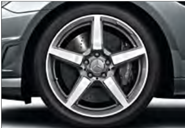
18" AMG 5-spoke alloy wheels, painted in Titanium Grey with burnished finish (standard on SLK 55 AMG, code 790)
