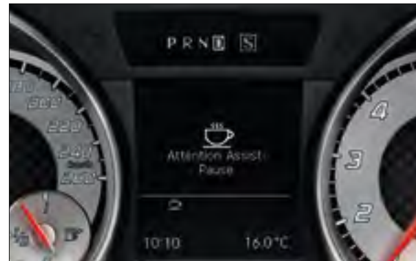
If it detects signs of tiredness or concentration lapses, Attention Assist suggests taking a break
