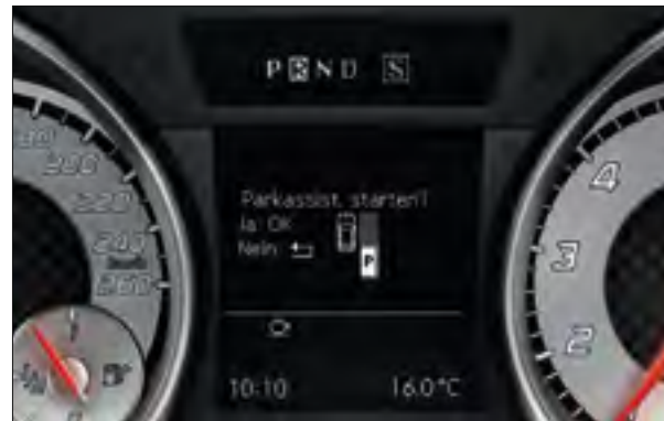
Parking Guidance identifies suitable parking spaces and helps you to manoeuvre safely in
