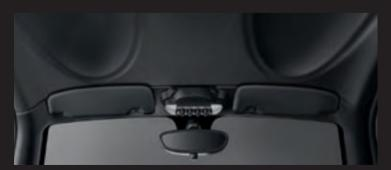
**Headliner in anthracite with ellipses.** The ceiling of the passenger compartment in the MINI Coupé comes as standard in this dark shade, and incorporates recesses in the same elliptical shape as the door trims. The result is more headroom and an uplifting sports-car feel. The controls for the interior lighting, the optional interior lights pack and the active rear spoiler are located above the rear-view mirror.
