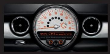
The large **speedo** in the middle of the instrument panel includes warning and indicator lights and the fuel gauge.
