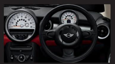
The **3-spoke sport leather steering wheel** also comes with multifunction controls as standard (optional for MINI Cooper Coupé and MINI Cooper Roadster). With this function, the cruise control, radio and telephone can be easily operated without removing the hands from the wheel.
