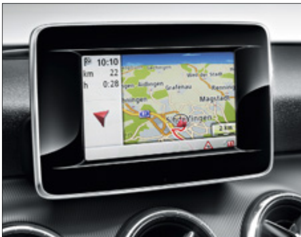
The Becker® Map Pilot navigation system works with the Audio 20 radio/single CD's display and the multi-function display in the instrument cluster
