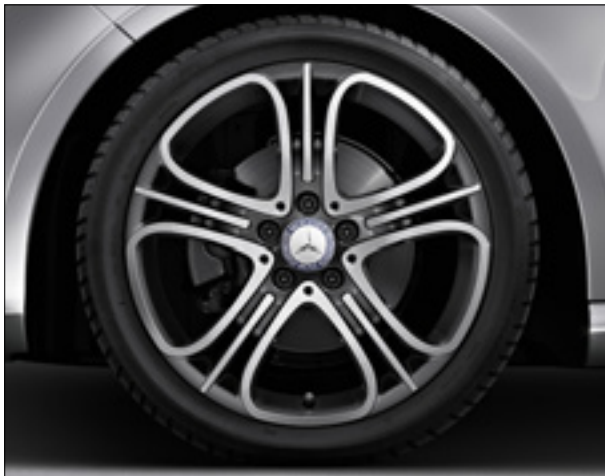
18" 5-triple-spoke alloy wheels in Tremolite metallic with 225/40 R 18 tyres
