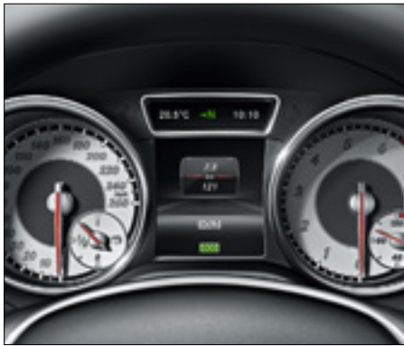
Instrument cluster in twin-tube design with colour LCD multi-function display
