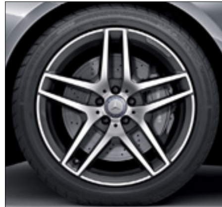
19" AMG 5-twin-spoke alloy wheels, burnished Titanium Grey finish, with 245/45 R 19 front and 275/40 R 19 rear tyres (standard on AMG Line, code 793)
