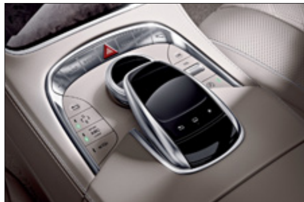
With the touchpad, telematic functions can be controlled conveniently with just one or two fingers
