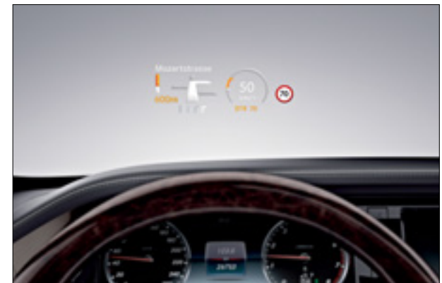
The head-up display shows important information directly in the driver's field of vision
