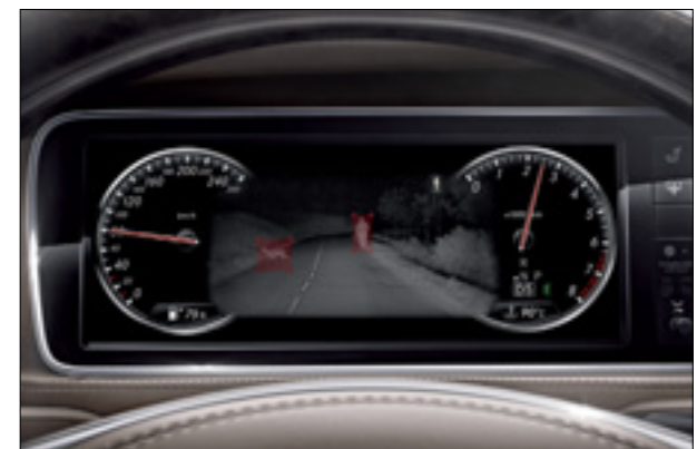
Night View Assist Plus displays detected pedestrians and helps the driver to react sooner to any potential danger
