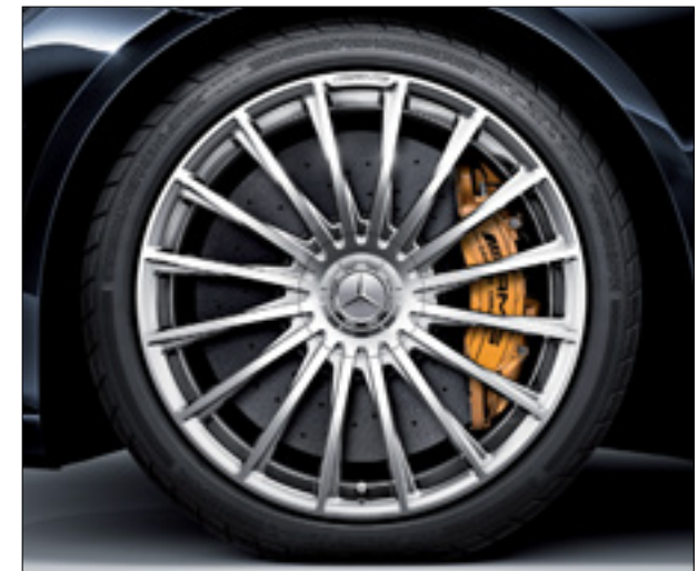
The standard 20" AMG multi-spoke forged wheels with optional AMG high-performance ceramic composite brake system
