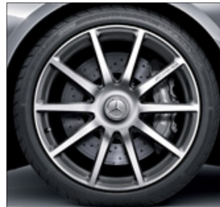
20" AMG 10-spoke forged wheels, polished Titanium Grey finish, with 255/40 R 20 front and 285/35 R 20 rear tyres (S 63 AMG L and S 65 AMG L, code 647)
