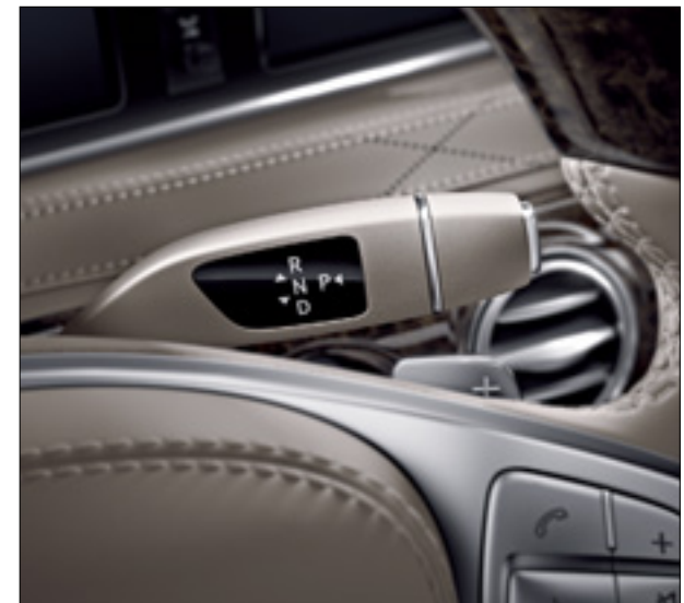
The Direct Select lever on the steering wheel. For manual gear changing, simply tap the gear shift paddles
