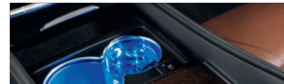
The cup holder with a heating and cooling function, identifiable by the red or blue colour.
