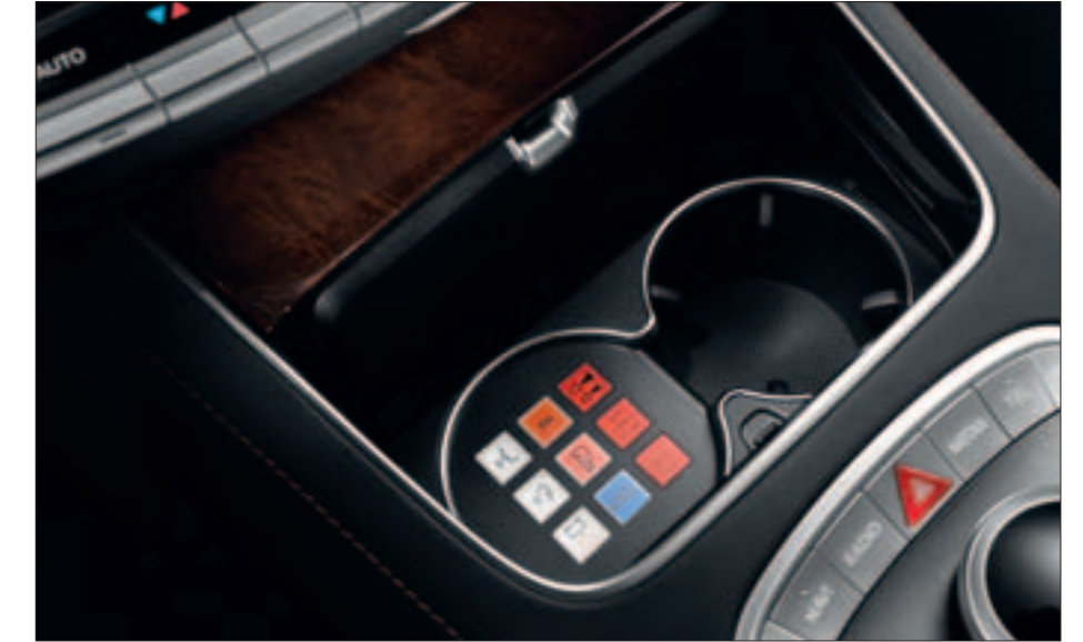
The activation button for the fire extinguishing system is marked clearly to ensure safe operation.
