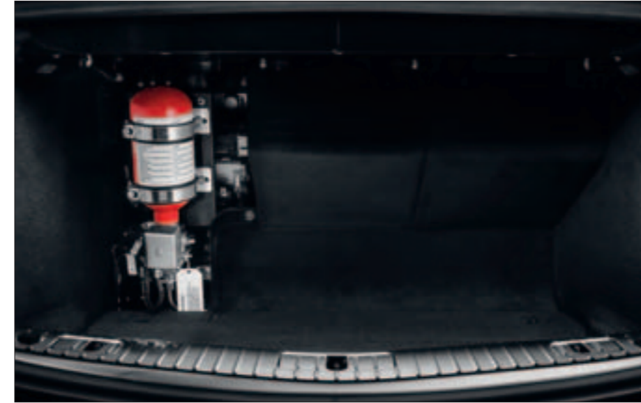
The bottle with the effective extinguishing agent is securely fastened in the boot.
