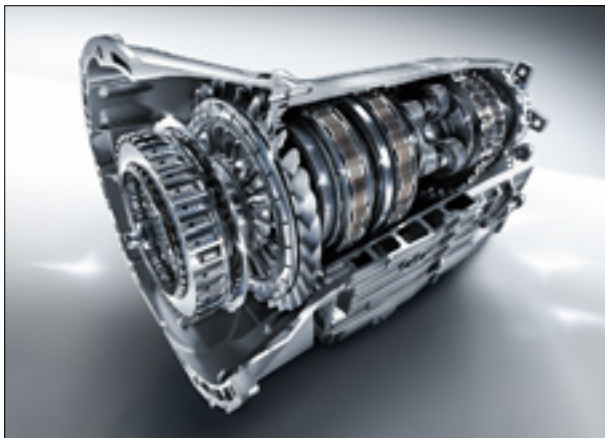
The SL 65 AMG is the first V12 Mercedes-Benz to feature AMG Speedshift Plus 7G-Tronic automatic transmission
