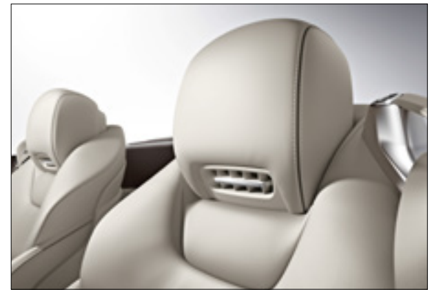
Airscarf neck-level heating system
