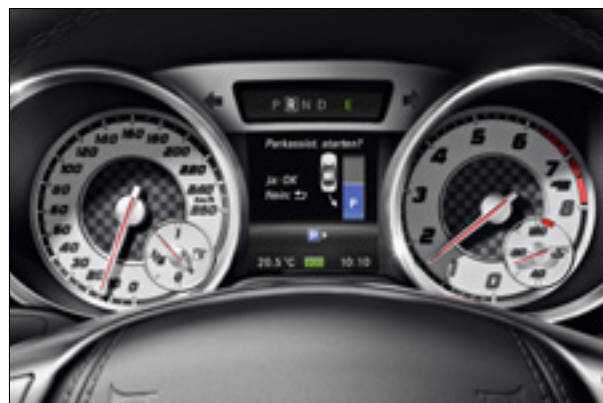
Active Park Assist identifies suitable parking spaces and can even steer you in automatically
