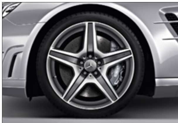
19" AMG 5-spoke alloy wheels, burnished Titanium Grey finish (standard on SL 65 AMG, code 797)
