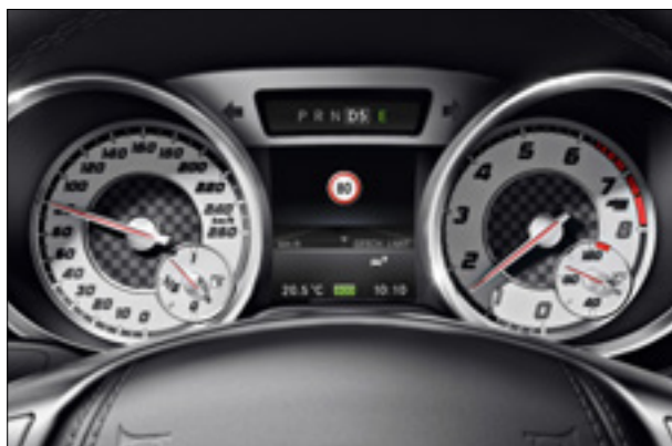
Speed Limit Assist shows you the current legal limit on the instrument panel and in COMAND Online's central display
