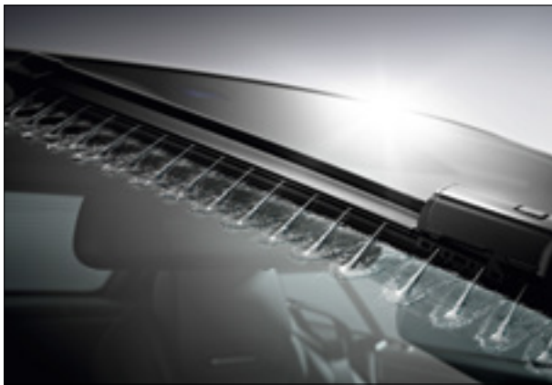
Magic Vision Control, the world's first adaptive windscreen wash system
