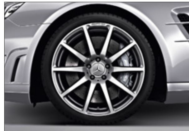
19"/20" forged AMG 10-spoke alloy wheels, polished Titanium Grey finish (optional on AMG models, code 766)
