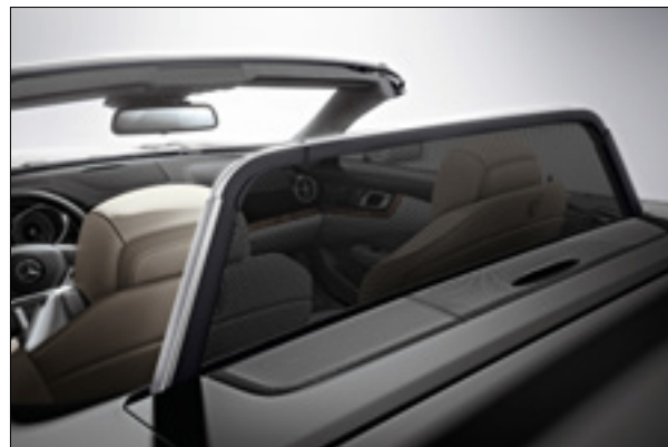
The electric wind deflector keeps draughts to a minimum in open-top driving
