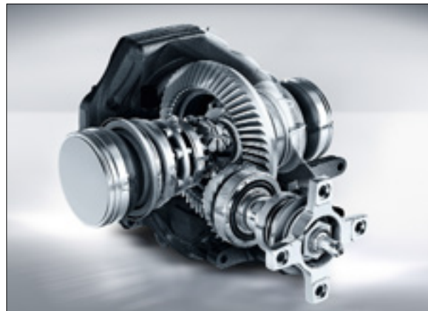
AMG rear axle locking differential with 40% locking effect
