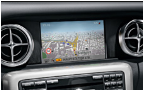
Speed Limit Assist shows the current speed limit in the instrument panel and in the central COMAND Online display
