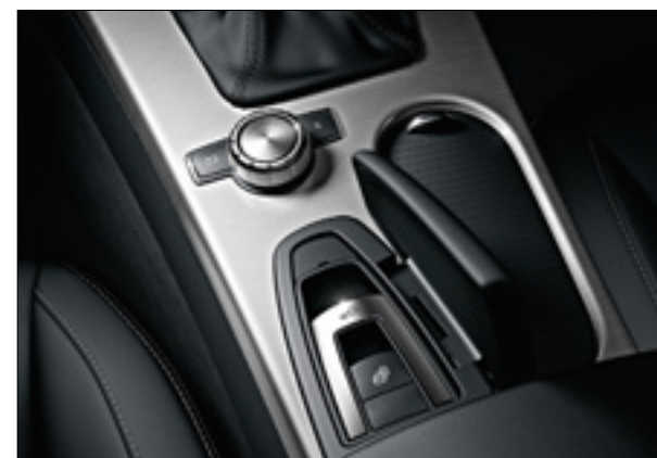
Roof controls and central controller
