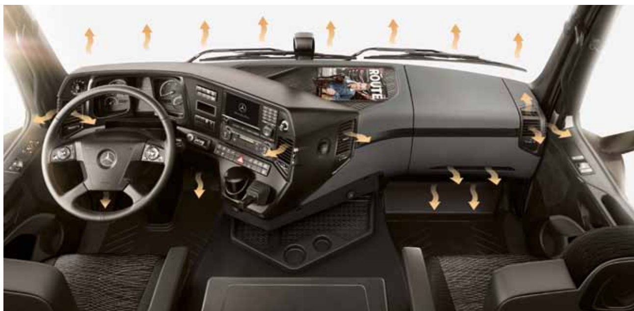
Heating, ventilation, climate. The Antos is equipped with a fast-acting air-controlled heating system. For even greater ease of use and comfort, an air conditioning system or an automatic climate control system can be specified. What's more, the residual engine heat utilisation system or various versions of the hot-water auxiliary heating system can maintain a pleasantly warm temperature during breaks, for example.
