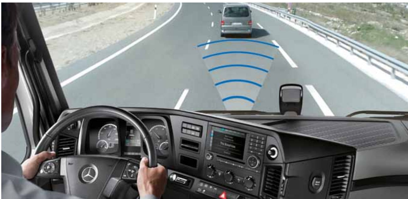
Proximity Control Assist 1) . The safety system with stop-and-go function is on hand to support the driver in stressful situations and reduces the risk of rear-end collisions. When approaching an identified vehicle driving ahead, the system reduces the speed and maintains the preset distance.
