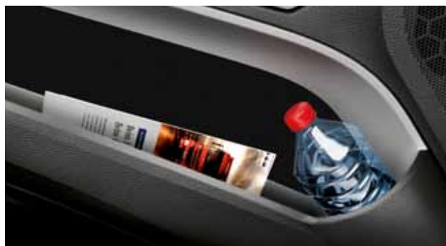
Door compartment. The stowage bins in the interior door trim offer space for items such as work gloves which should be kept within easy reach without having to climb into the cab. Each one also incorporates a bottle holder large enough for a 1.5 l bottle.
