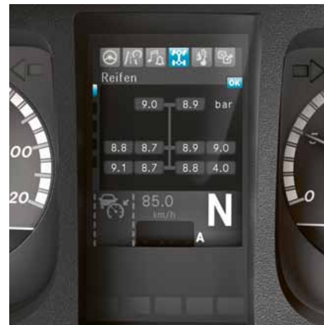
Tyre pressure monitoring system 2) . The wireless pressure monitoring system for the front and rear axles continuously monitors the air pressure in all the tyres of the tractor unit as well as those of the semitrailer or trailer.
