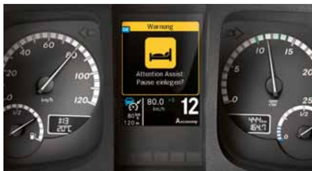
Attention Assist 2) . The system can recognise increasing tiredness and recommend the driver takes a break.
