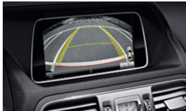
The optional reversing camera supports static and dynamic guidelines in reversing operations
