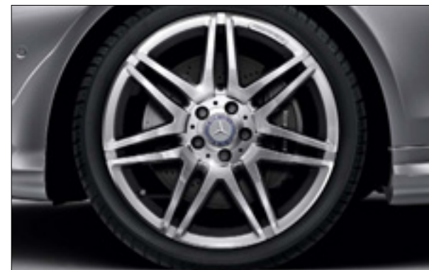
19" AMG 7-twin-spoke alloy wheels, with front 235/35 R 19 and rear 255/30 R 19 (optional on AMG Line, code 770)
