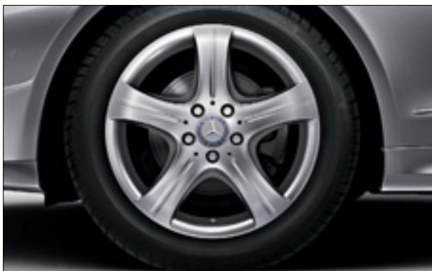
17" 5-spoke alloy wheels with front 235/45 R 17 and rear 255/40 R 17 tyres (optional on SE, code R22)
