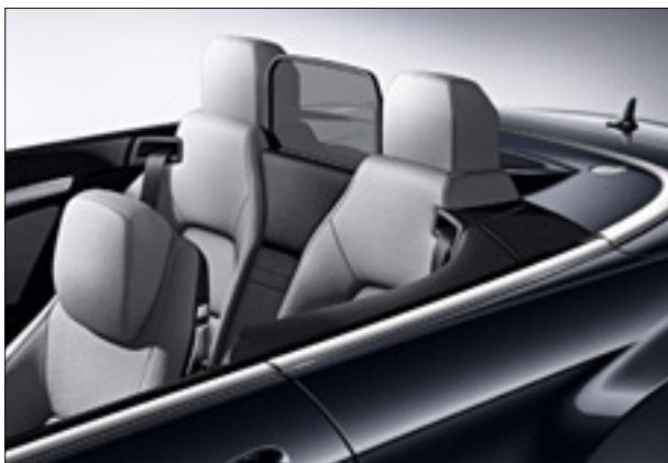
Roll bars integrated into the head restraints of the rear seats (Cabriolet only)
