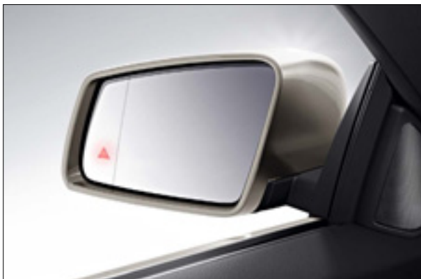
Lane-Keeping Assist and Blind Spot Assist can alert the driver in potentially dangerous situations; for example, when changing lanes
