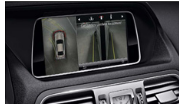
The central display of the COMAND Online system shows the area around the vehicle during parking
