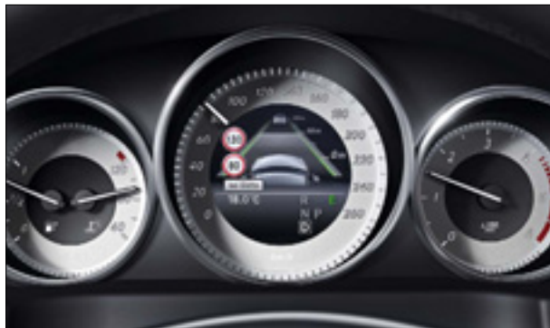
Traffic Sign Assist shows the driver what speed limits and traffic signs apply
