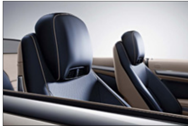
The Airscarf heating system wraps around the front passengers' necks like a scarf
