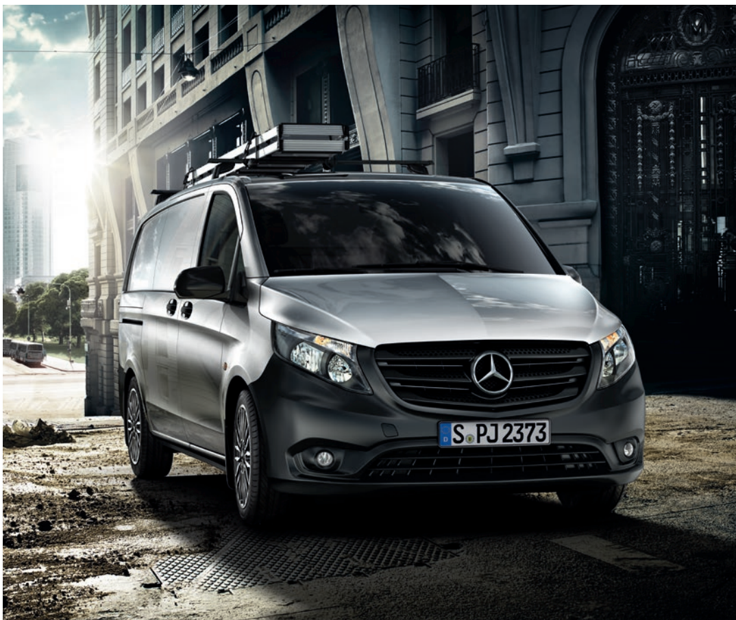
Standard basic carrier bars, two crossbars. Set of 2 basic carrier bars for models with standard roof. Screw-fit to designated points in roof channel. Adding an optional 3rd crossbar increases maximum permissible roof load from 100kg to 150kg. Usable width: 135cm.
