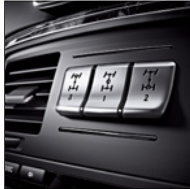
Sequentially lockable differentials
