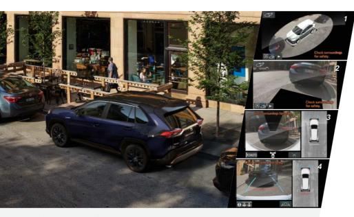
When reverse parking, the smart rear-view camera shows you when to turn the steering wheel. It also displays your path, based on the wheel's position.
