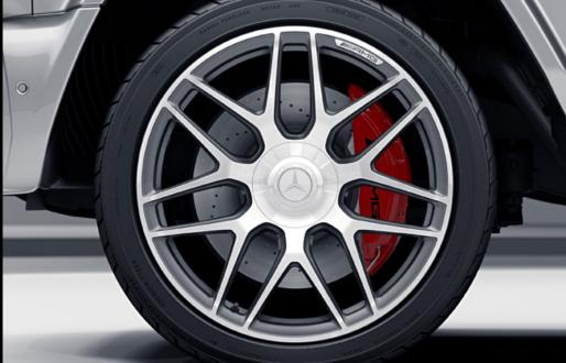
RG5 22" AMG forged wheels - cross-spoke design, painted titanium grey with a high-sheen finish, 295/40 R 22 tyres
