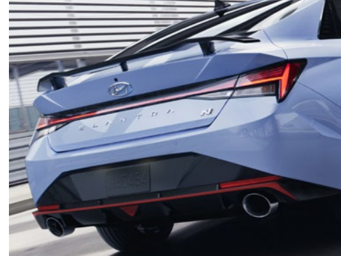
Wing-type rear spoiler N rear bumper and diffuser Variable exhaust valve system with dual outlets
