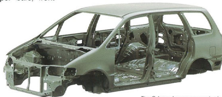
The Odyssey's monocoque body provides a strong flex-resistant platform.
