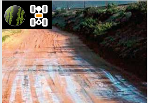
4HLC (4WD High Range with locked centre differential) For rugged terrain with low-grip surfaces.*
