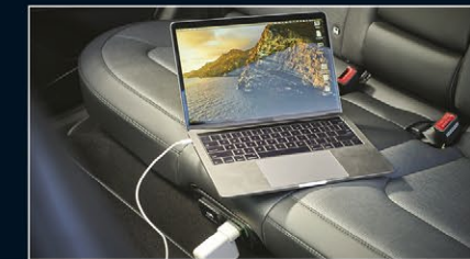
Vehicle to Load Interior Socket (EV Standard)
