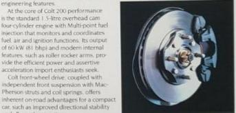
Colt sport suspension system for DOHC GT models uses heavy duty coil springs and an antisway har in front and rear plus gas-charged rear shock absorbers
