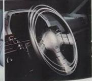
The tilt and selescope steering wheel standard on 200 CT DOHC and on 200 LX and 200 SX 4-door sedans, assumes that every driver can select a comfortable position.
