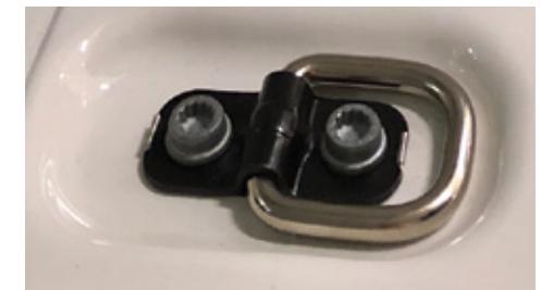
The lashing eyes are recessed to lie flush with the floor.
